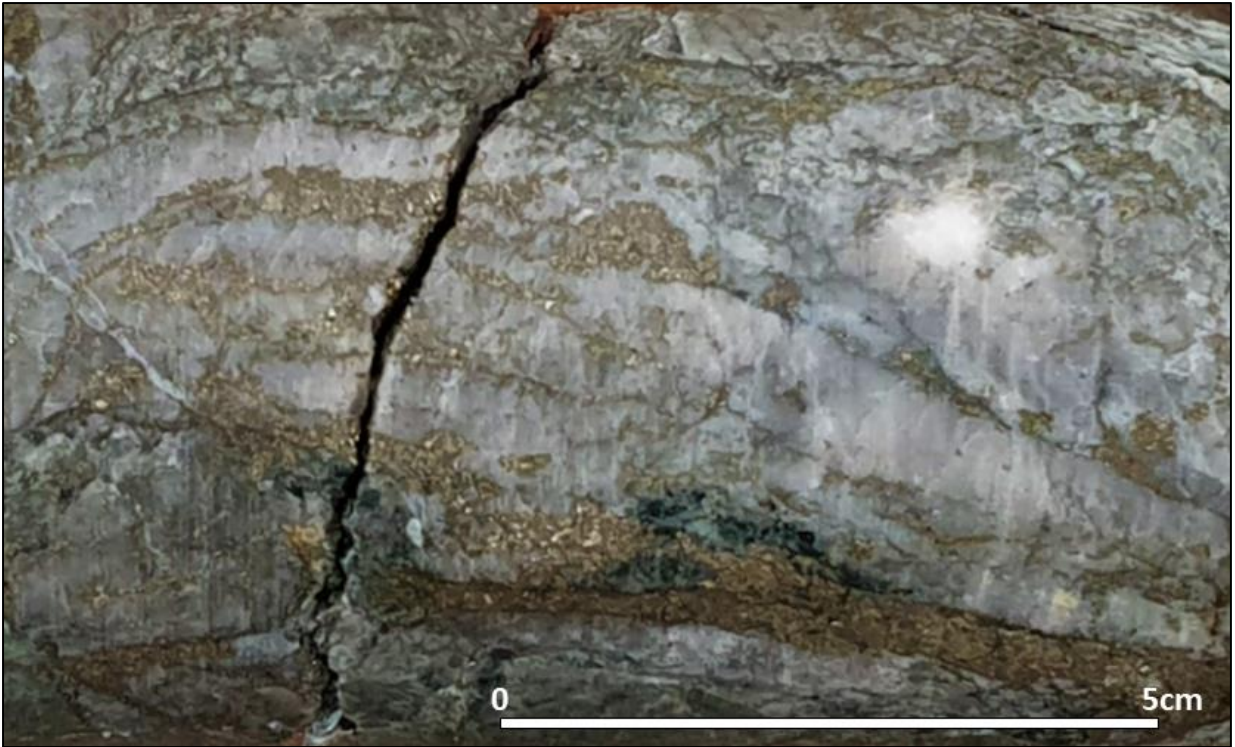
Figure 4: Selected drill core example of visible chalcopyrite-pyrite mineralization, including trace visible bornite, at 68.8m depth in TAD-20-002.
