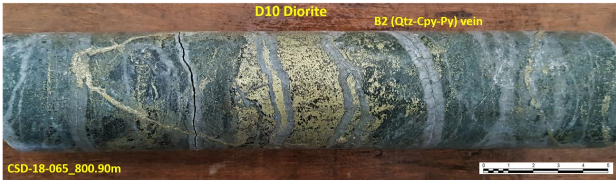
Figure 3: Core photo from Hole CSD-18-065 showing the intersection of a D10 Diorite containing moderate Act-propylitic alteration overprinted by weak Argillic alteration.
