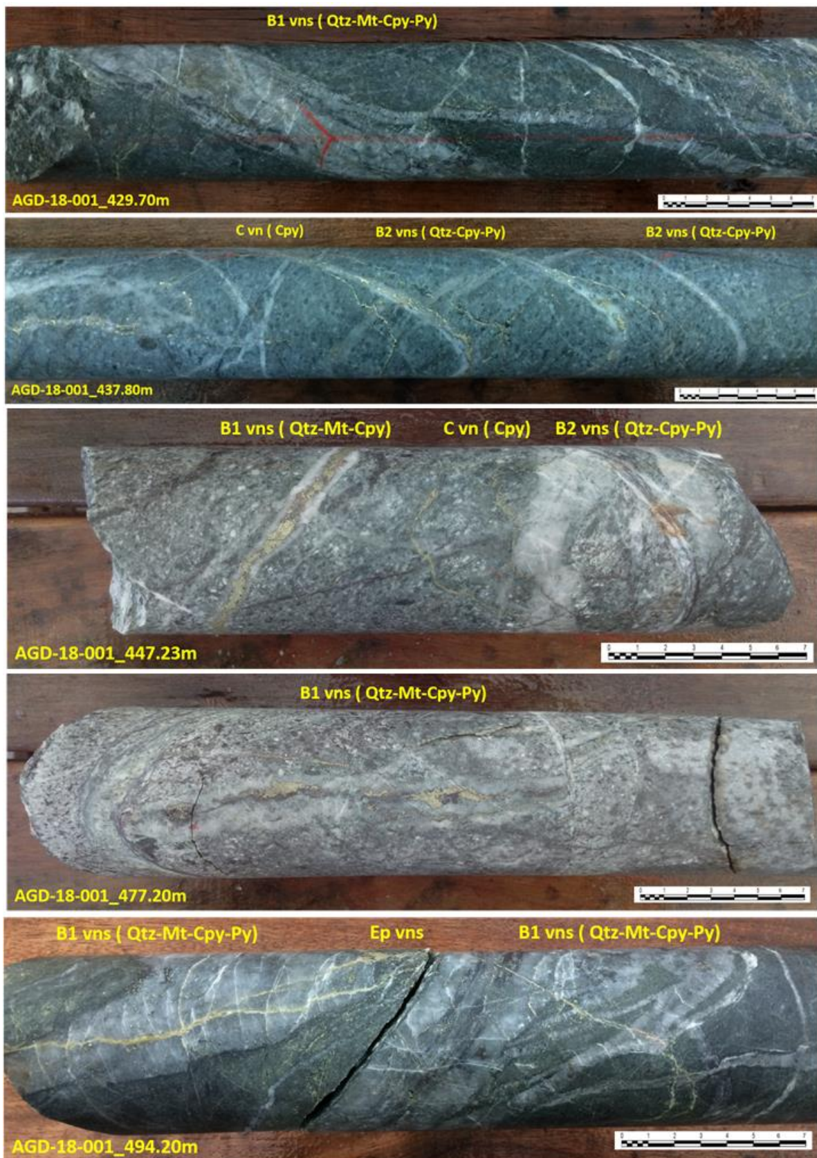
Figure 4: Selected examples of mineralization observed in Aguinaga drill hole AGD-18-001 to date.
